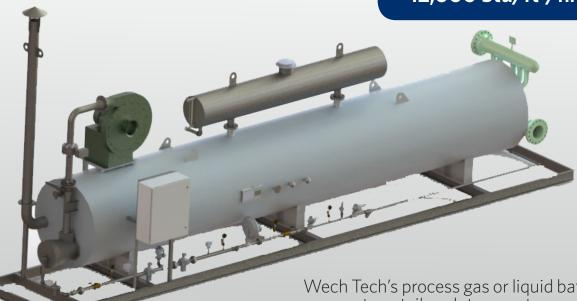
Wech Tech's process gas or liquid bath heating systems are custom-tailored to meet your temperature and pressure requirements. Each system is designed with a fire tube and exhaust stack, process coil, and water saver tank. The line of bath heating systems are safe and cost effective with a life span average of 20+ years.
